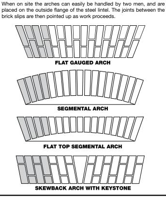
**Prefabricated Brick Arches** Our prefabricated brick arches are made by cutting standard bricks to either voussoirs or skewbacks, then into brick slips. The brick slips are then bonded with an epoxy resin onto a composite lightweight
